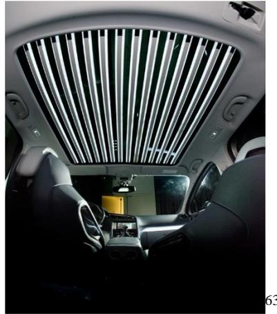
Another innovation from PSA used in the Chrysalide Concept is the Cielo Magic light. The light comes from a sticker on the sunroof which displays a desired pattern of reflection on the inside. This technique gives the impression of a real light source.<sup>64</sup>
