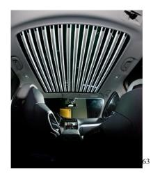
Another innovation from PSA used in the Chrysalide Concept is the Cielo Magic light. The light comes from a sticker on the sunroof which displays a desired pattern of reflection on the inside. This technique gives the impression of a real light source.<sup>64</sup>
